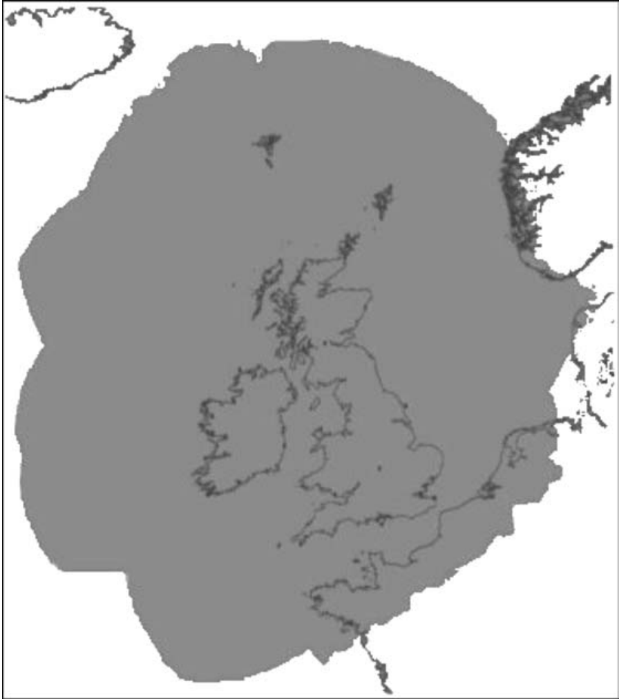
Figure 1. Daytime service availability provided by the 16 beacons of the United Kingdom and Ireland. Light grey = 99.8%, Dark grey = 99.5%.
