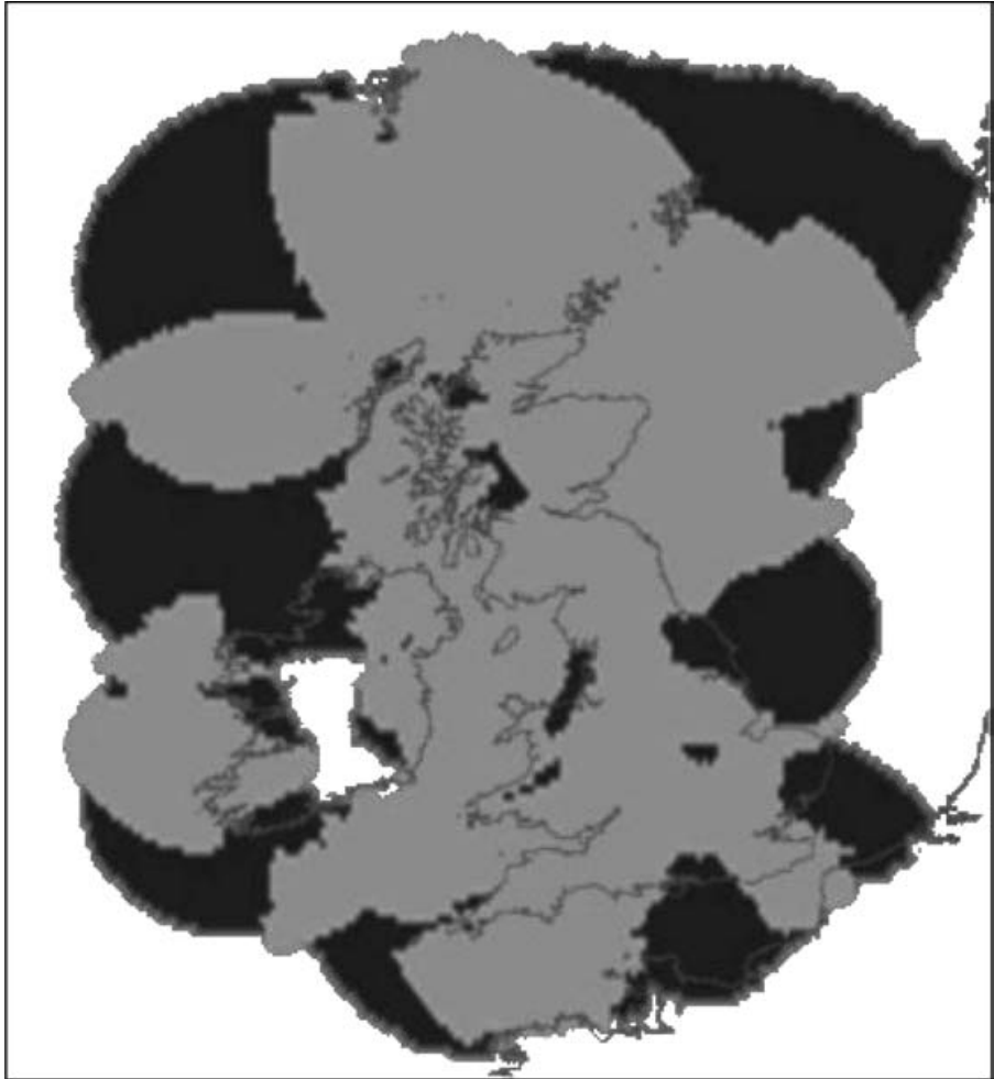
Figure 3. Two-year service availability provided by the 16 beacons of the United Kingdom and Ireland. Light grey=99.8%, Dark grey=99.5%.
