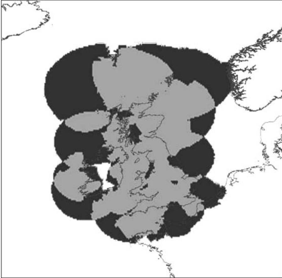
Figure 9. Night-time 3-hour service continuity for the 16 beacons of the UK and Ireland. Light grey = 99.97% (critical areas requirement met), Dark grey = 99.85% (other areas requirement met).
