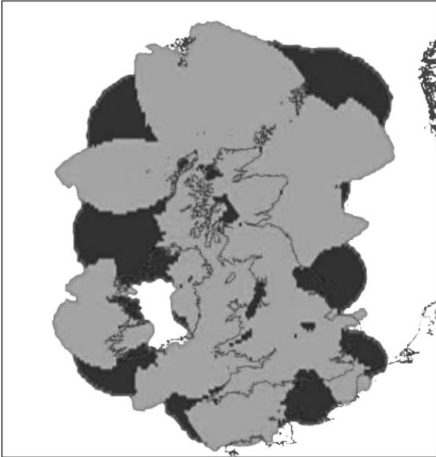
Figure 12. Night-time service meets coverage, availability and continuity requirements. Light grey=99-97% (critical areas requirement met), Dark grey=99-85% (other areas requirement met).
