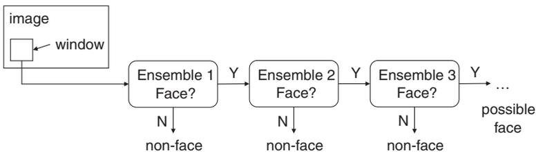
**FIGURE 6.14** Operation of the cascade face detector.
