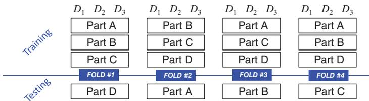
FIGURE 5.17 Standard 4-fold cross-validation set-up.
