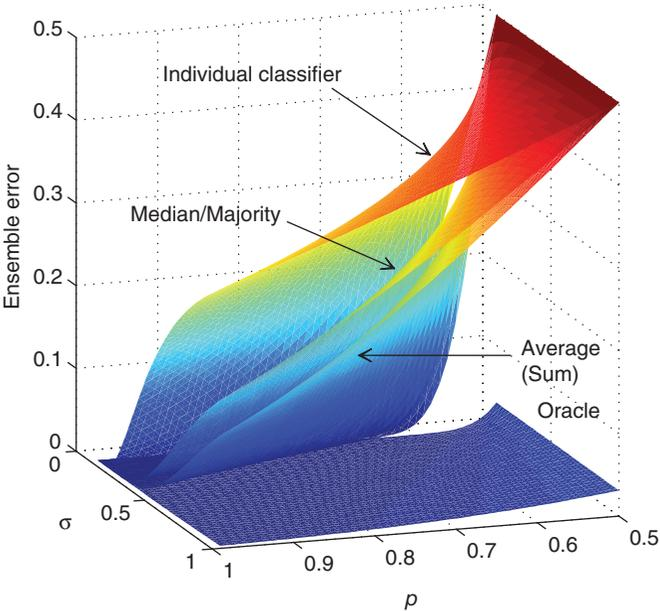
**FIGURE 5.9** Ensemble error rate of the individual classifier and the simple combiners for normal distribution of the estimation error  $\eta$ .
