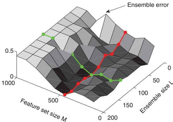
**FIGURE 9.12** RS error on the real fMRI data set as a function of the ensemble size  $L$  and the feature size  $M$  [225].
