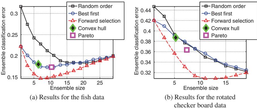
**FIGURE 8.15** Averaged testing errors from 50 runs of the five overproduce-and-select methods.
