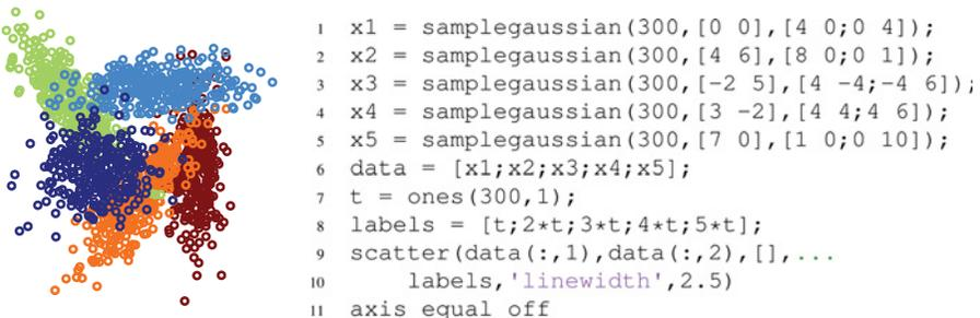
**FIGURE 1.6** An example of five Gaussian classes generated using the `samplegaussian` function from Appendix 1.A.1.
