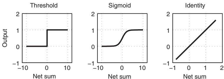
**FIGURE 2.13** Threshold, sigmoid, and identity activation functions.
