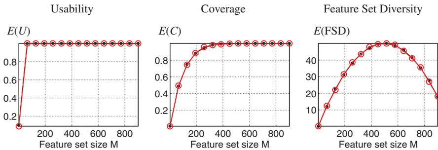
**FIGURE 9.11** Theoretical and simulation curves (coinciding) for the expected values of  $U$ ,  $C$ , and  $FSD$  for  $n = 1000$ ,  $Q = 100$ , and  $L = 10$ . The empirical curve is calculated as an average of 10 ensembles with randomly sampled  $L = 10$  sets of  $M$  features.
