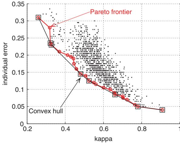
**FIGURE 8.14** An example of the convex hull and Pareto frontier of an ensemble cloud in a kappa-error diagram.
