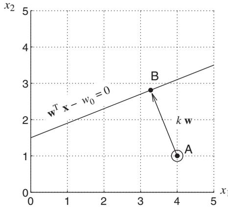
FIGURE 2.17 Illustration of the distance calculation from  $A$  to the line.
