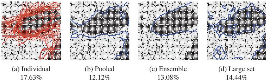
**FIGURE 2.24** Boundaries of 1-nn classifiers. The values underneath are the error rates with respect to the noise-free data.
