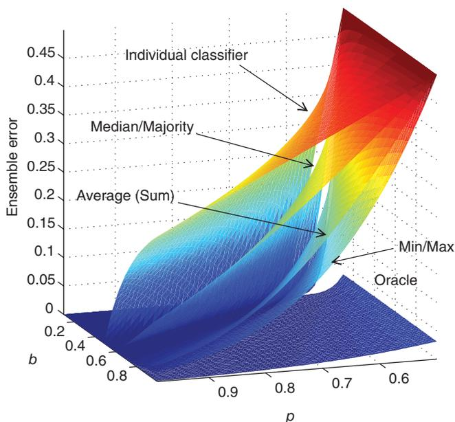
**FIGURE 5.10** Ensemble error rate of the individual classifier and the simple combiners for uniform distribution of the estimation error  $\eta$ .
