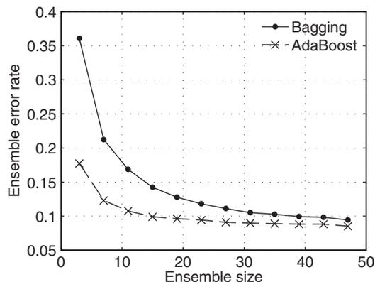
**FIGURE 6.7** Testing error of AdaBoost and bagging versus the ensemble size for the fish data set.
