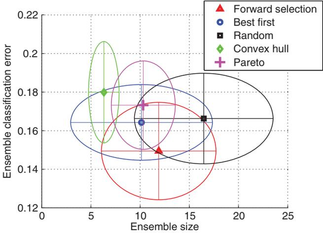
**FIGURE 8.16** Results with the fish data. Ensemble size and testing error for the five overproduce-and-select methods, averaged across 50 runs. The ellipses mark one standard deviation of the points from the mean.
