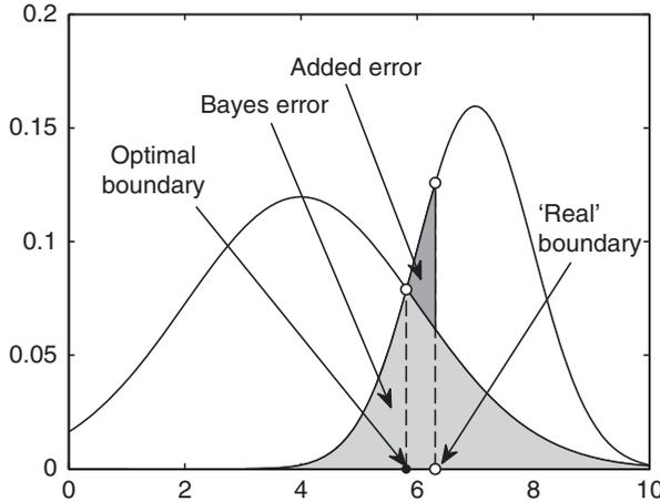
**FIGURE 1.19** Plot of two discriminant functions  $P(\omega_1)p(x|\omega_1)$  (left curve) and  $P(\omega_2)p(x|\omega_2)$  (right curve) for  $x \in [0, 10]$ . The light-gray area corresponds to the Bayes error, incurred if the optimal decision boundary (denoted by  $\bullet$ ) is used. The dark-gray area corresponds to the additional error when another boundary (denoted by  $\circ$ ) is used.
