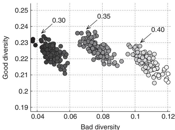
**FIGURE 8.9** 300 ensembles of  $L = 7$  classifiers in each one. The oracle outputs were generated independently, with probability of classification error as indicated. The gray-level intensity signifies the majority vote error. Lighter color corresponds to larger error.
