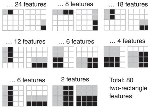
**FIGURE 6.13** The two-rectangle Haar-like features for a window of size  $4 \times 4$ .
