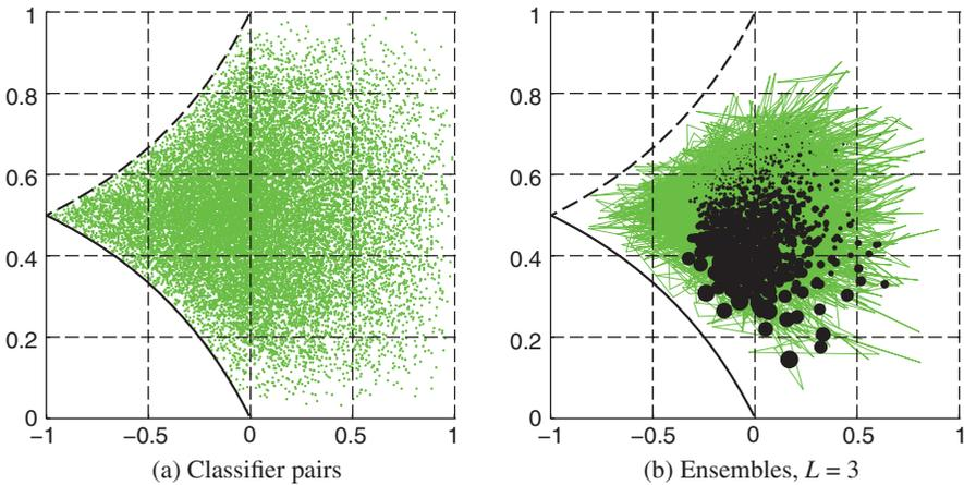
**FIGURE 8.11** Illustration of the bound of the kappa-error diagram. (a) 20,000 pairs of classifiers; (b) ensembles of three classifiers, where larger marker indicates higher accuracy.
