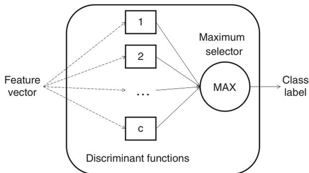
**FIGURE 1.9** Canonical model of a classifier. An  $n$ -dimensional feature vector is passed through  $c$  discriminant functions, and the largest function output determines the class label.
