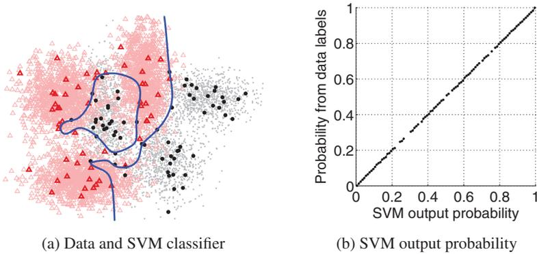
**FIGURE 5.2** Calibrated output for the SVM classifier on a two-dimensional two-class data set.
