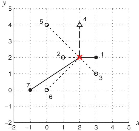
**FIGURE 5.3** A point in a two-dimensional feature space and its seven nearest neighbors from  $\omega_1$  (open circles),  $\omega_2$  (bullets), and  $\omega_3$  (triangle).
