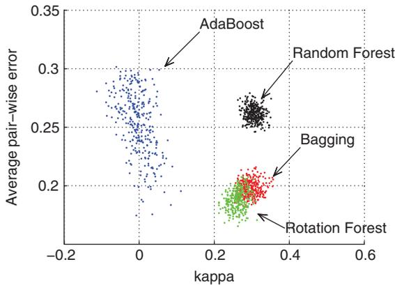
**FIGURE 8.10** A kappa-error diagram of four ensemble methods for the letter data set. Testing errors: AdaBoost 5.76%, bagging 9.46%, random forest 9.26%, and rotation forest 8.47%.
