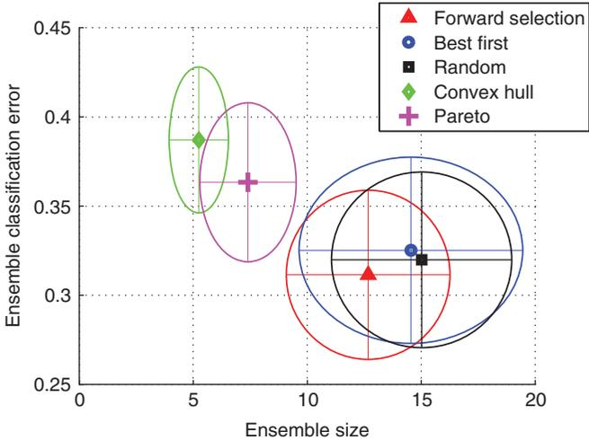
**FIGURE 8.17** Results with the rotated checker board data. Ensemble size and testing error for the five overproduce-and-select methods, averaged across 50 runs. The ellipses mark one standard deviation of the points from the mean.
