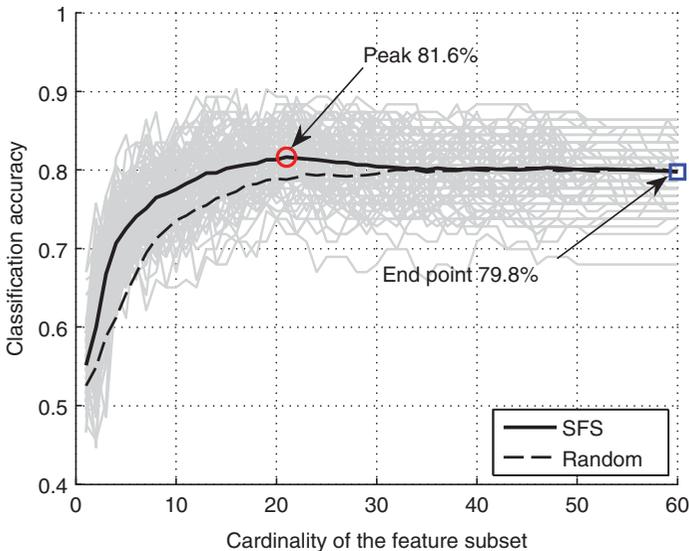
**FIGURE 1.24** Illustration of the peak effect in feature selection on the “sonar” data, SFS filter and the nearest neighbor classifier.
