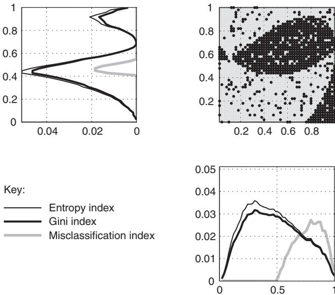
**FIGURE 2.6** Three indices of impurity used in growing decision trees: entropy-based, Gini, and misclassification, calculated for 50 split points for each of  $X$  and  $Y$  for the fish data set.
