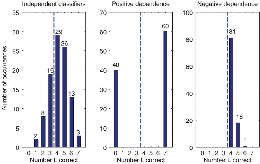
**FIGURE 8.3** Patterns of difficulty for three classifier ensembles with  $L = 7$ ,  $p = 0.6$ , and  $N = 100$ . The dashed line is the majority vote border. The histograms show the number of points (out of 100) which are correctly labeled by  $i$  of the  $L$  classifiers. The  $x$ -axis shows the number of correct classifiers.
