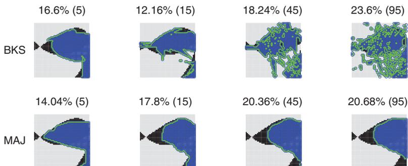
**FIGURE 6.22** Classification regions for the RLO and the NB classifier. Two combination methods were tried: BKS (top row) and majority vote (bottom row), for different ensemble sizes as shown in the brackets. The ensemble error rate is shown in the plot titles.
