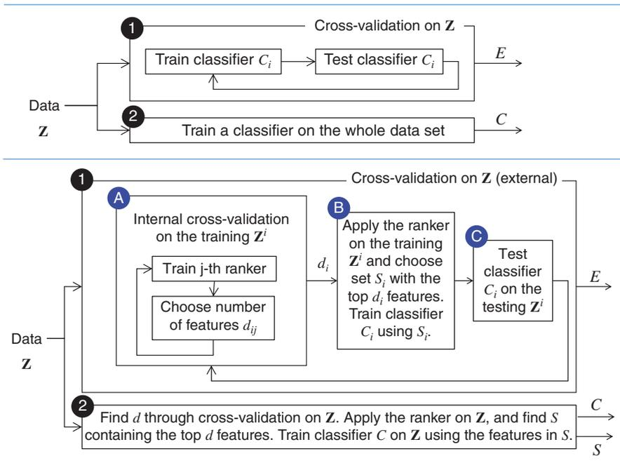
**FIGURE 9.2** An example of a noncontaminated experimental protocol for feature selection and classification.
