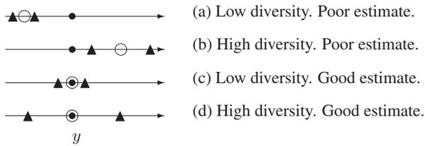
**FIGURE 8.1** Examples of low and high diversity for a point-value estimation.  $\bullet$ —true value  $y$ ;  $\circ$ —estimate  $\hat{y}$ ;  $\blacktriangle$ —estimator outputs.
