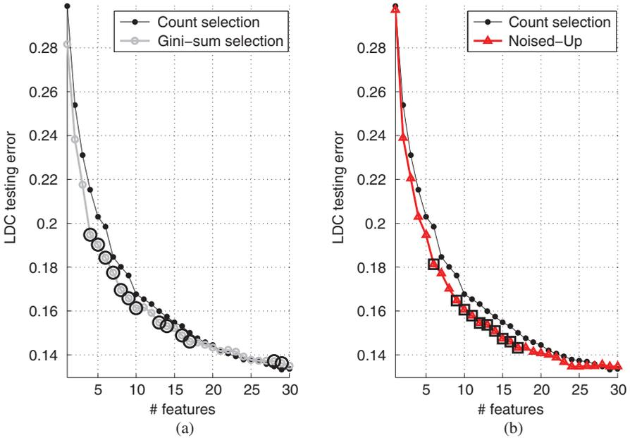
**FIGURE 9.8** Results from the sign rank test between the count ranker and: (a) the Gini-sum ranker; and (b) the noised-up ranker. The points where significant difference was found are marked with circles (a) and squares (b).
