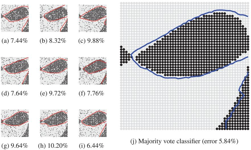
**FIGURE 3.3** (a)–(i) Classification boundaries of nine MLP classifiers trained on the fish data set with 10% label noise. Displayed underneath each plot is the testing error. (j) Boundary of the majority vote ensemble classifier.
