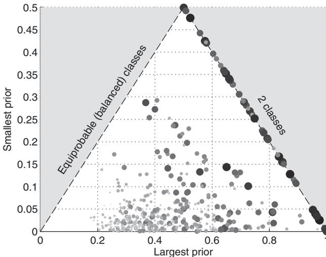
**FIGURE 2.25** The triangle diagram. The size and the gray-level intensity of the dots indicate the classification accuracy. Larger and darker dots signify higher accuracy.
